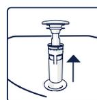
1 Lift the water trap from the waste outlet.
